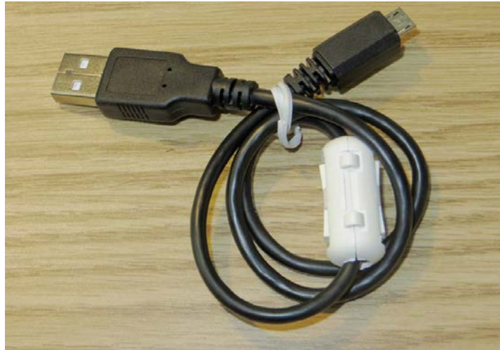
USB Cable used for testing w/ ferrite added to pass radiated immunity
