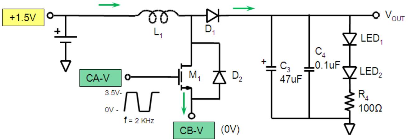
Figure 6, measuring the switch current
