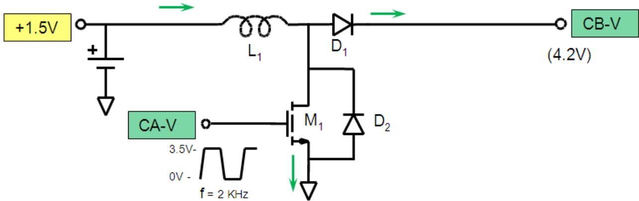
Figure 4, measuring the diode current.
