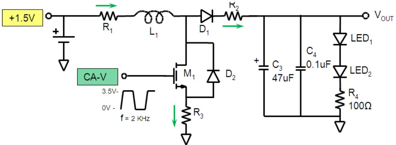
Figure 1, DC-DC Boost converter with current shunt resistors.
