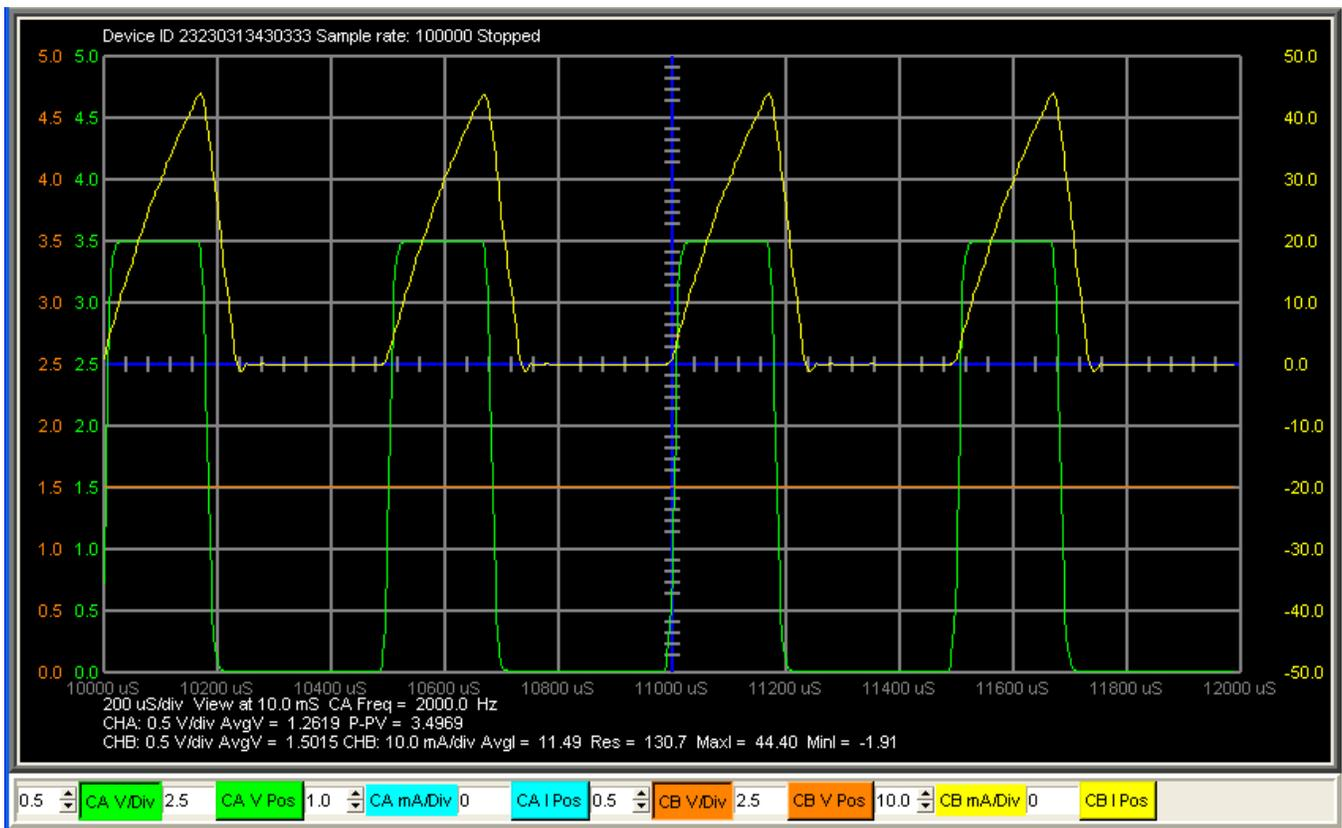
Figure 3, Inductor current waveform
