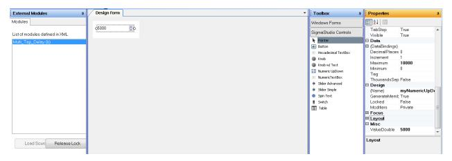
Click Multi\_Tap\_Delay in *Modules*, then set pin names to "Input Signal", "Delay Tap", and "Delayed Input" accordingly. Their sequence is derived from the XML file.
