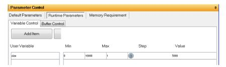
The next step is to connect the "Numeric UpDown" widget to the created variable "size". Click mouse right button on the "Numeric UpDown" widget in the Design Form. Choose <u>Assign</u> and you should see a similar window shown below. Set Control Action to CheckedChanged and Run-Time Parameter to the variable, enable. Click Apply.
