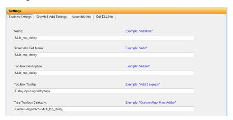
This module is created with one input channel, one delay control tab and one output channel. If we allow the module to grow more channels, we should configure it in "Growth & Add Settings", as shown below. The number of delay control taps and delay outputs can go up as many as four pairs or down as few as one pair.
