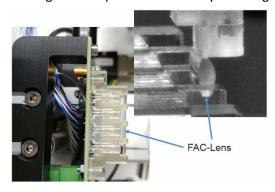
these lenses requires a custom lens holder and also active lens alignment fitting during the manufacturing process. This was done at FISBA [2], a worldwide leading supplier of customized optical components, systems and microsystems with locations across Europe and in the US.
