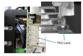
the seglents of customines afcustom lens holder and also active lens alignment fitting during the manufacturing process. This was done at FISBA [2], a worldwide leading supplier of customized optical components, systems and microsystems with locations across Europe and in the US.
