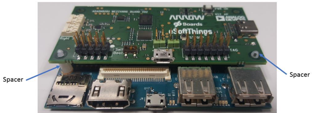
Figure 14: Assembly Mezzanine and DragonBoards
