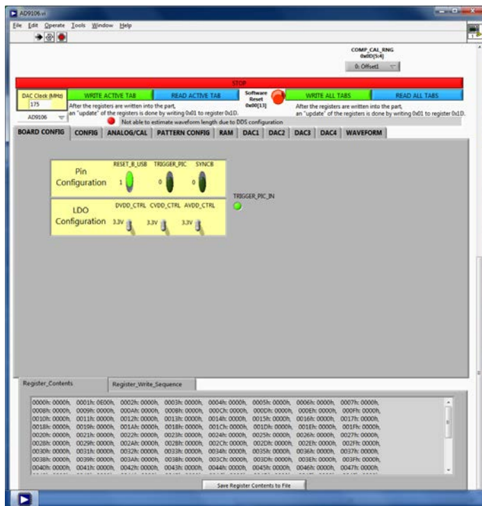
Figure 1: AD9106 evaluation software Control Panel GUI, Board Configuration Tab
