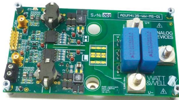
Figure 1. ADuM4135 Gate Drive Module
